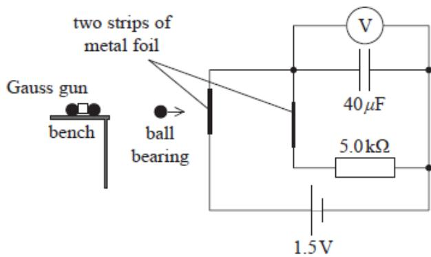
As the ball bearing left the gun, it broke the first foil strip at its centre so that the capacitor started to discharge. When the ball bearing broke the second foil strip the capacitor discharge stopped.
