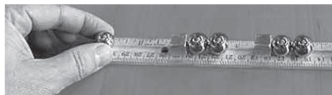
Pairs of ball bearings are placed to the right of two strong magnets. A single ball bearing is released from the left, as shown. The ball bearing is attracted to, and collides with, the first magnet. This and all subsequent collisions can be assumed to be elastic.
