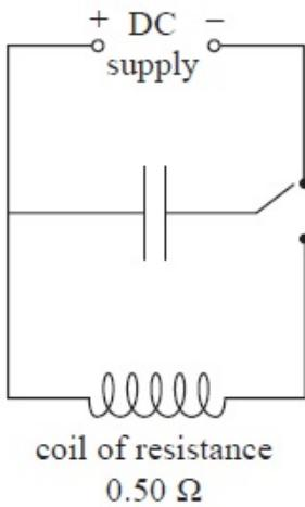
The circuit contains a capacitor of capacitance  $600 \mu\text{F}$ . This capacitor is suitable to provide the current for  $1.4 \times 10^{-3} \text{ s}$ .
