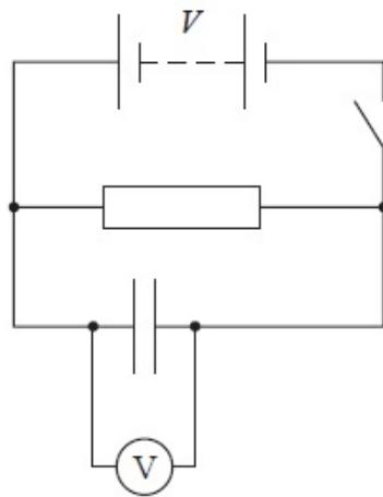
The switch is opened and the p.d. across the capacitor allowed to fall. A short time later the switch is closed again. Select the graph that shows how the p.d. across the capacitor varies with time, after the switch is opened.
