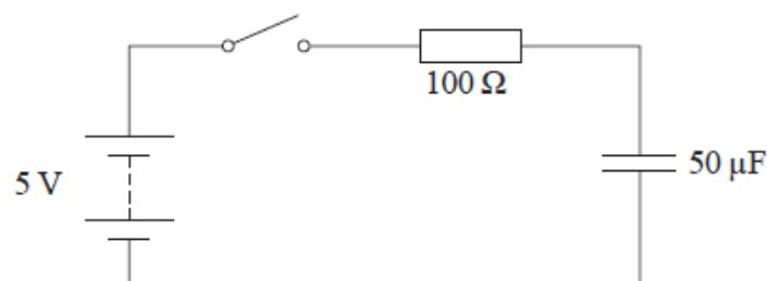
Describe what happens to the potential difference across the resistor and the potential across the capacitor after the switch is closed.
